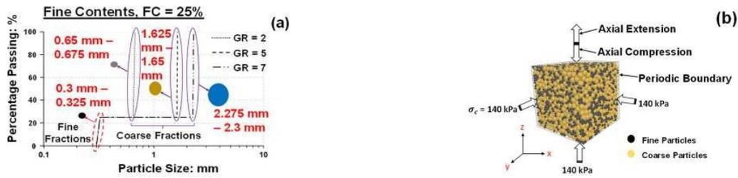
Figure 1. (a) Particle-size distribution curve for varying gap-ratios, (b) DEM sample.
